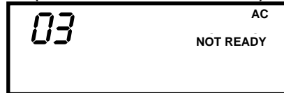
TYPICAL DISPLAYS INDICATING FAULTED PROTECTION ZONE (AFTER PRESSING READY KEY)
